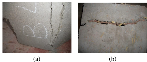
Fig. 7 – Graphical representation of bridging effect of concrete specimens with (a) Sisal fiber reinforced plaster; and (b) Rice straws reinforced plaster [123].
