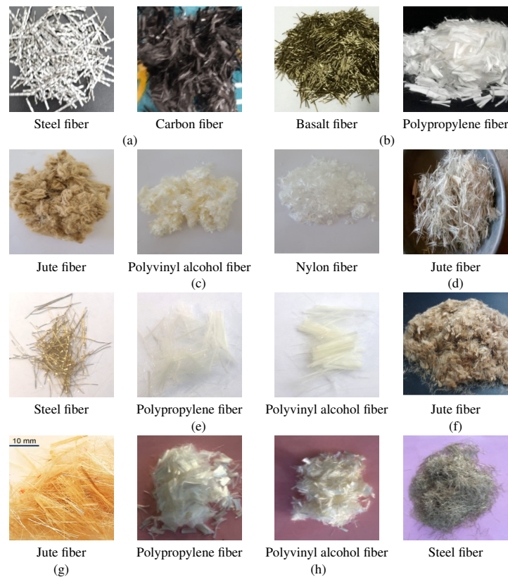
Fig. 1 – Various hybrid fibers and single fiber used in cementitious materials: (a) Steel fiber and Carbon fiber [15]; (b) Basalt fiber and Polypropylene fiber [16]; (c) Jute fiber, Polyvinyl alcohol fiber and Nylon fiber [17]; (d) Jute fiber [18]; (e) Steel fiber, polypropylene and polyvinyl alcohol [19]; (f) Jute fiber [20]; (g) Jute fiber [21]; (h) Polypropylene fiber, Polyvinyl alcohol fiber and Steel fiber [22].
