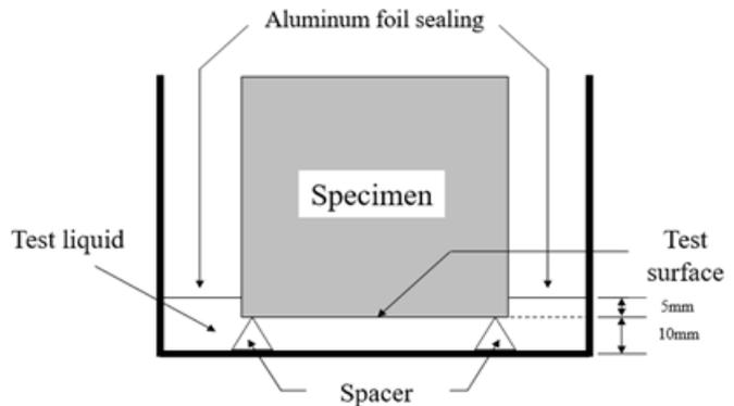
(b) Specimen of de-icing salt scaling test
