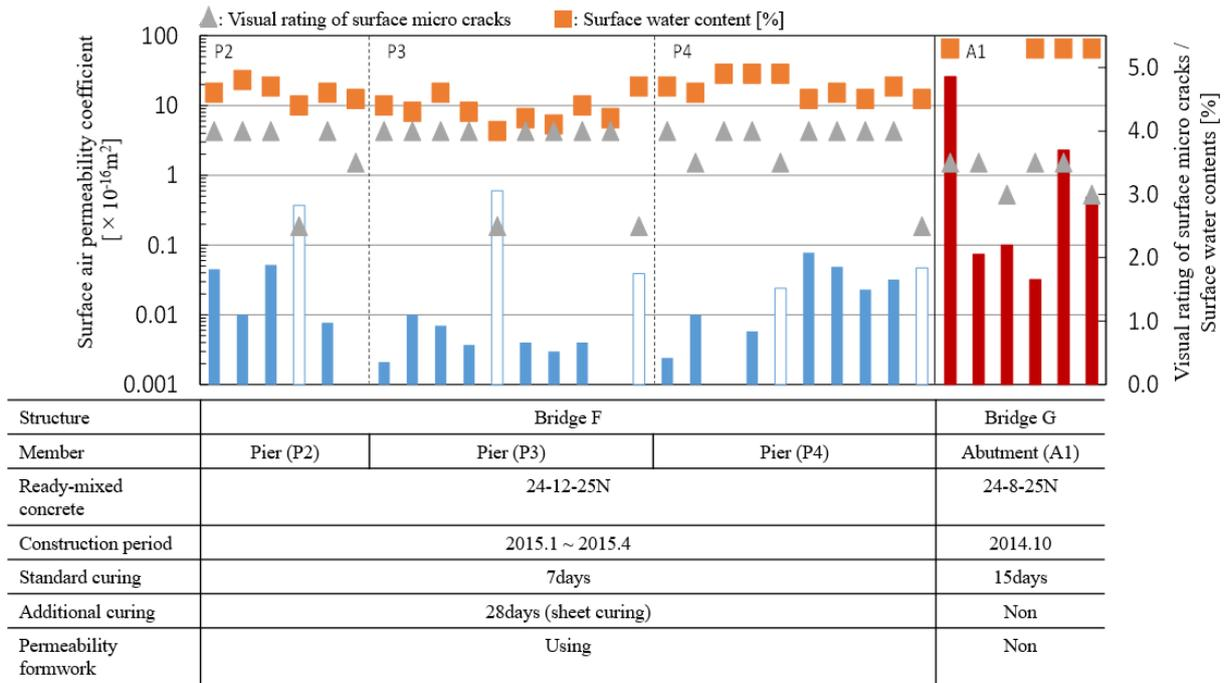
Fig. 5 – Effect of the permeability formwork on the surface air permeability of structure
