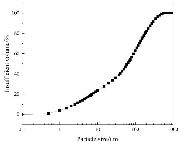
Fig. 4 – Distribution of tailings particle size
