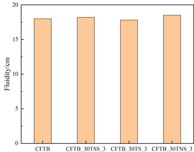
Fig. 8 – Changes in backfill fluidity under the action of different activators
