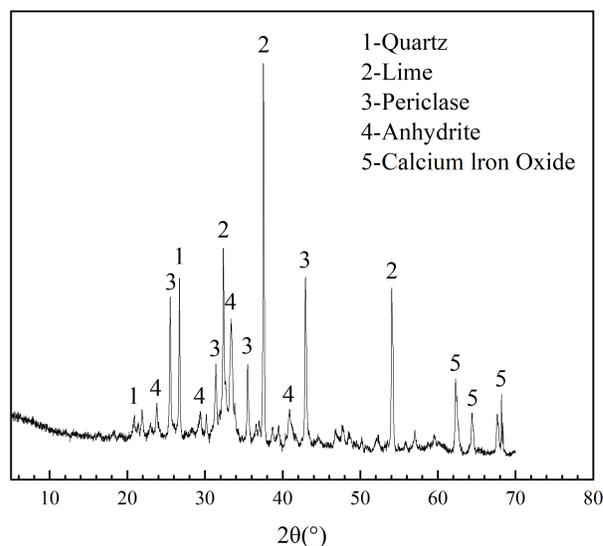
Fig. 2 – Mineral composition of fly ash
