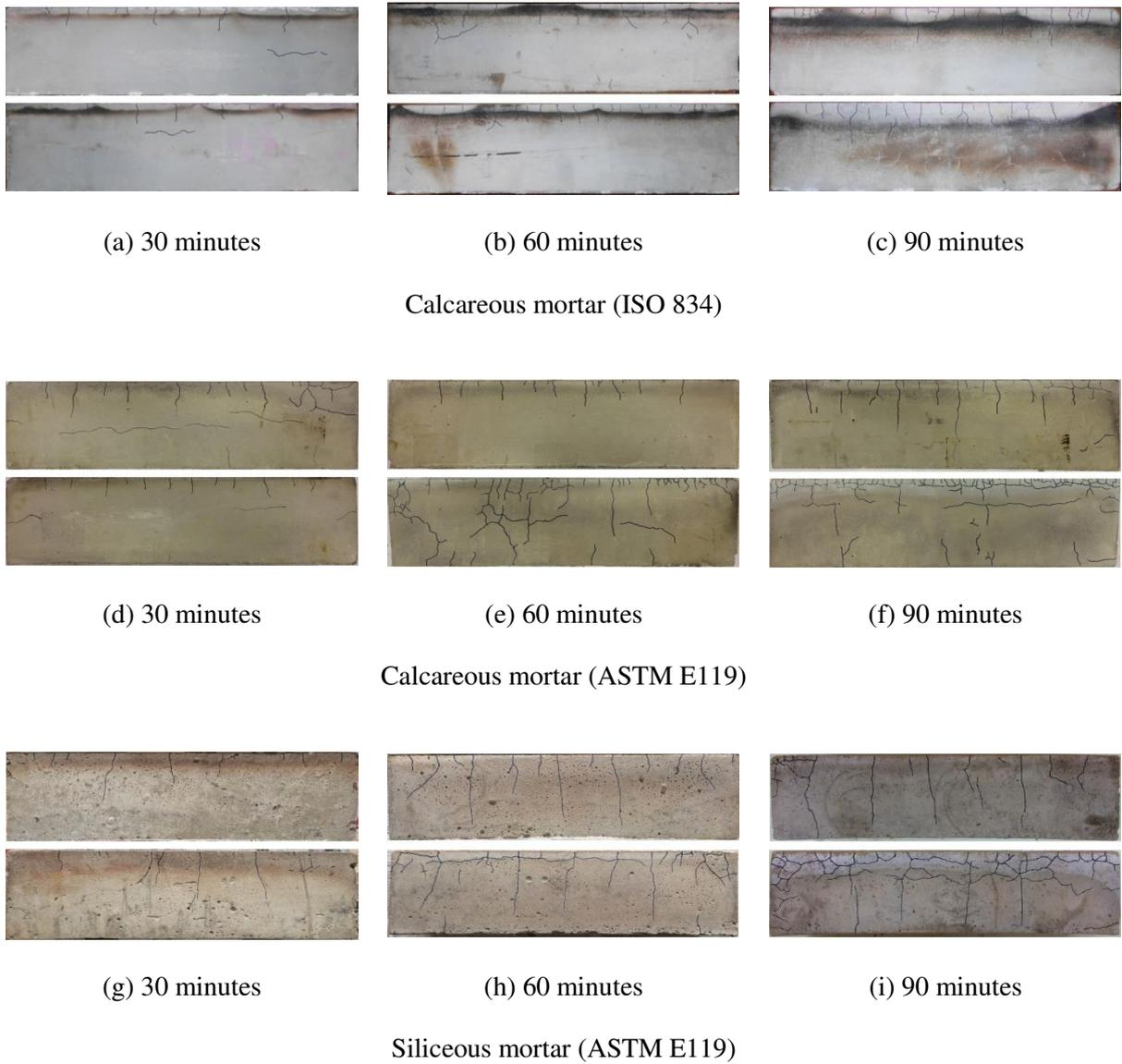
Fig. 7 – Crack patterns on both sides of specimens
