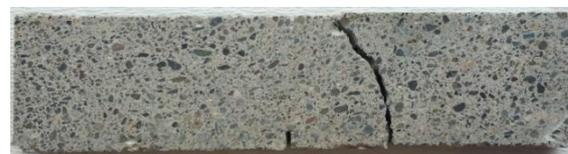
(b) For specimen with existing fire crack
