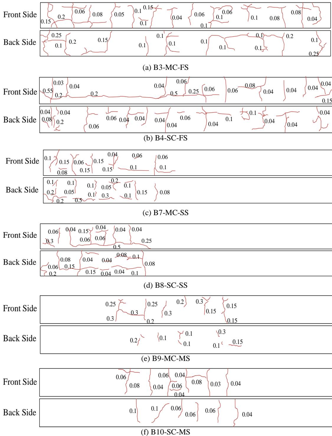
Fig. 7 – Corrosion crack widths and distributions of corroded beams
