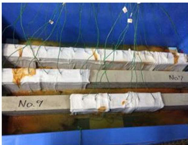
Fig. 2 – Corrosion process for beams
