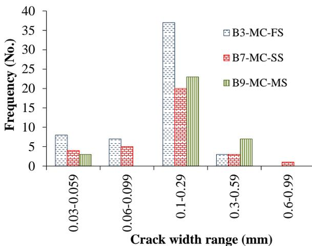
Fig. 5 – Corrosion crack width frequencies for mild corrosion
