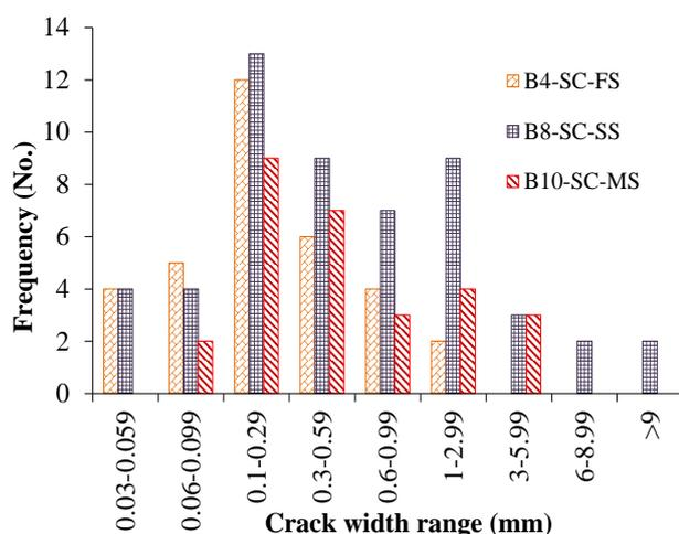
Fig. 9 – Flexural crack width frequencies for severe corrosion
