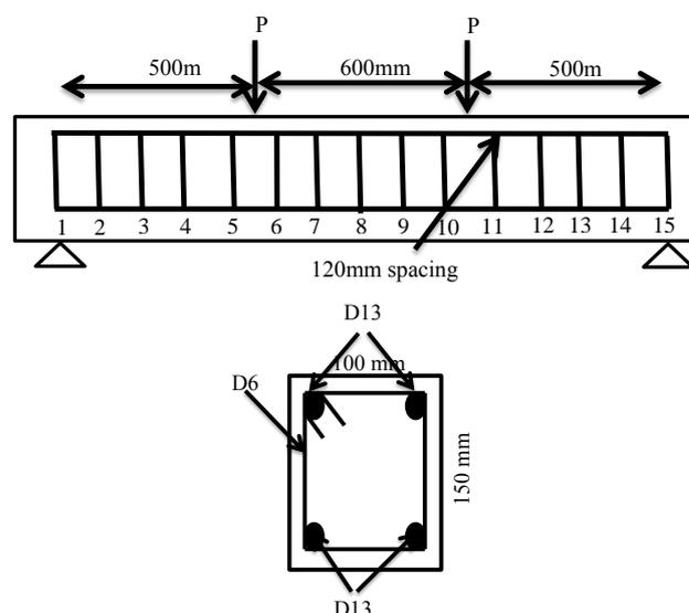
Fig. 1 – Beam layout and cross sectional view
