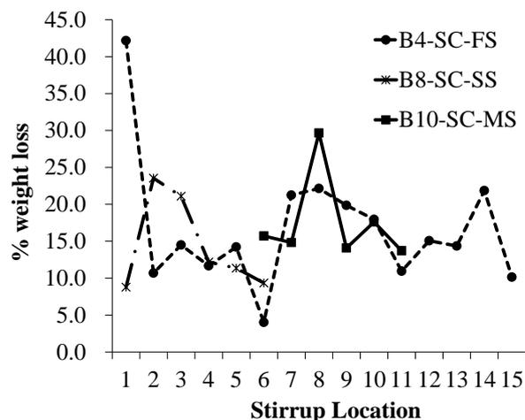
Fig. 4 – Weight loss of stirrups for severe corrosion
