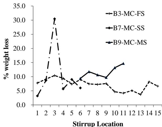
Fig. 3 – Weight loss of stirrups for mild corrosion
