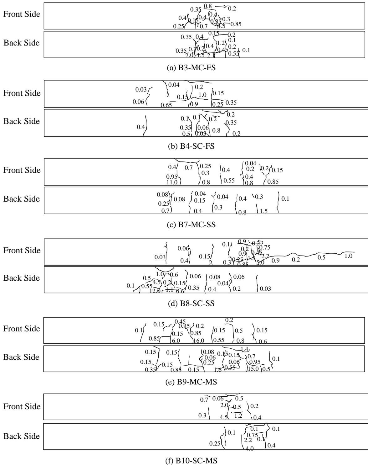
Fig. 10 – Flexural crack widths and distributions of corroded beams
