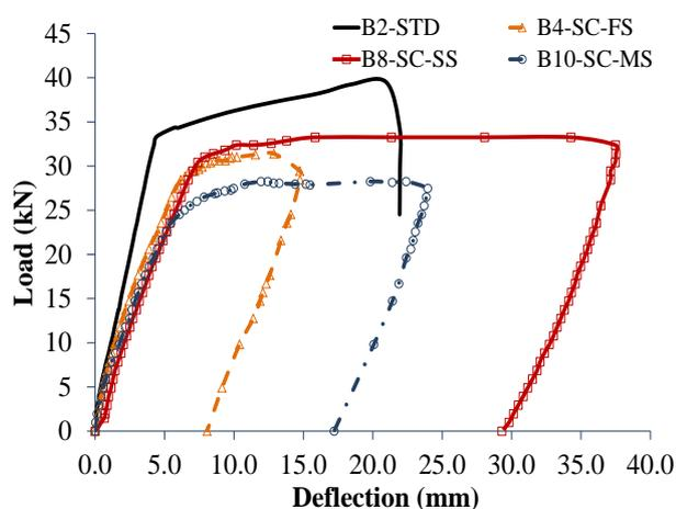
Fig. 12 – Load-deflection curves for severe corrosion
