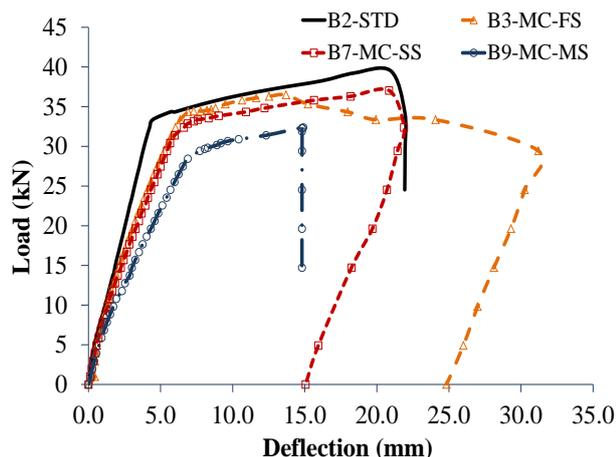
Fig. 11 – Load-deflection curves for mild corrosion
