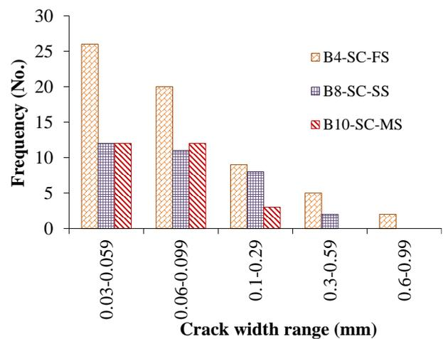
Fig. 6 – Corrosion crack width frequencies for severe corrosion
