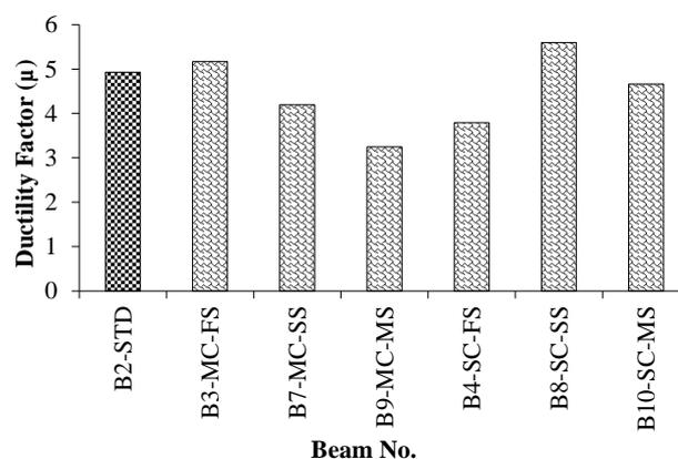
Fig. 13 – Deflection ductility factor of the corroded beams
