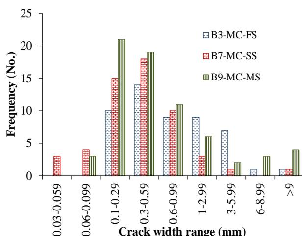
Fig. 8 – Flexural crack width frequencies for mild corrosion
