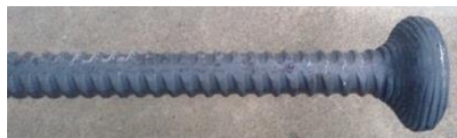
Fig. 1 – Mechanical anchorage: headed reinforcement
