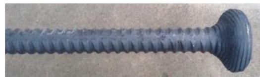
Fig. 1 – Mechanical anchorage: headed reinforcement
