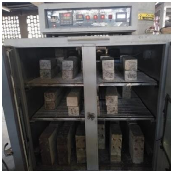
Fig. 4 – Accelerated carbonation resistance test
