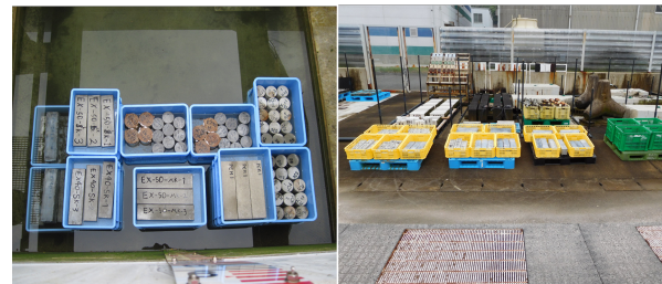
Photo 2 Exposure conditions of the various specimens (Submerged zone and Tidal and splash zone)
