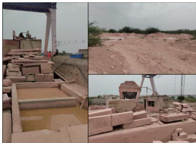
Fig. 1 Dimensional stone waste generation at the factory stage (Bayana village in Rajasthan)
