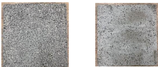
(a) Cast surface (b) Formwork bottom surface
