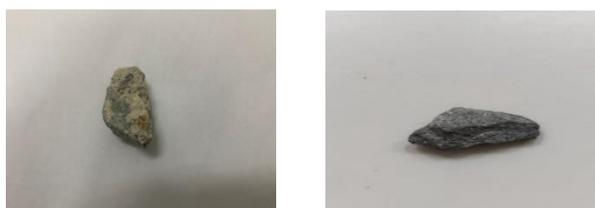
(a) Recycled aggregate      (b) Natural aggregate
