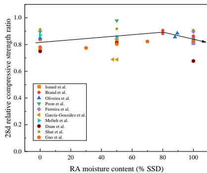
(c) The relationship between the moisture content of RA and the 28d relative compressive strength of RAC
