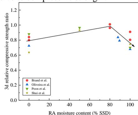
(a) The relationship between the moisture content of RA and the 3d relative compressive strength of RAC
