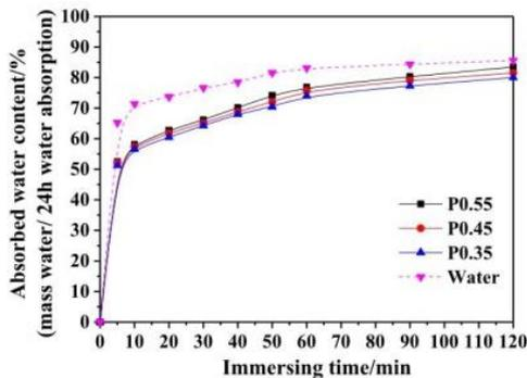
(c) R2 time-varying water absorption in cement paste
