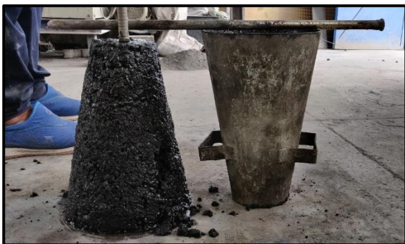
Fig. 3: 'Workability of pervious concrete
