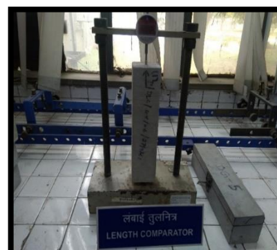
Fig. 5 – Test set up for evaluation of drying shrinkage of concrete beam specimen
