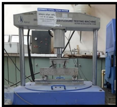
Fig. 2 – Test set up for evaluation of flexural strength of concrete beam specimen
