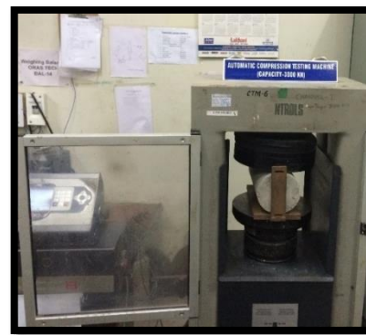
Fig. 3 – Test set up for evaluation of split tensile strength of cylindrical concrete specimen
