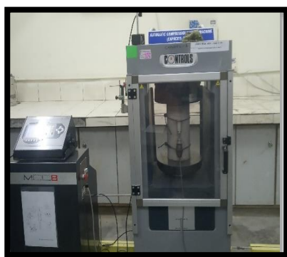
Fig. 4 – Test set up for evaluation of Modulus of Elasticity and Poisson's ratio of concrete specimen
