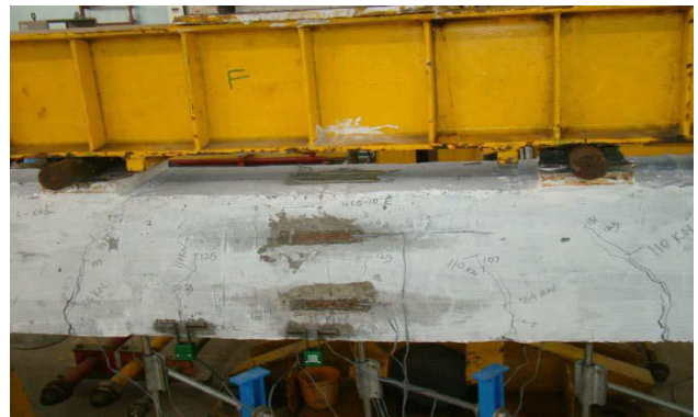
(f) final cracking at ultimate load
