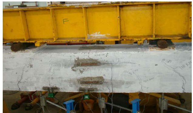
(h) final cracking at ultimate load
