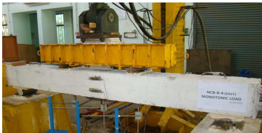
Fig. 3 – Flexural strength testing arrangement for PSC beams
