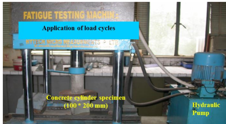
Fig. 5 – Fatigue testing arrangement
