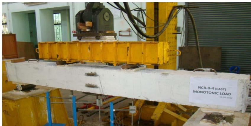
Fig. 3 – Flexural strength testing arrangement for PSC beams
