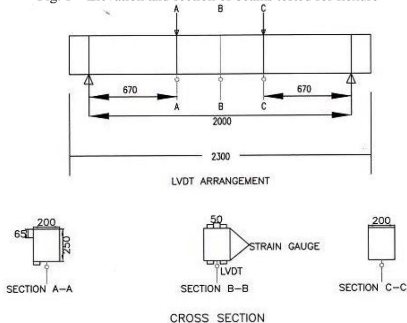
Fig. 2 – Testing setup along with instrumentation details
