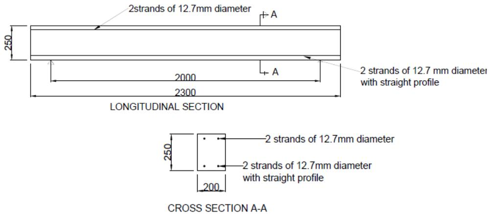
Fig. 1 – Elevation and section of beams tested for flexure
