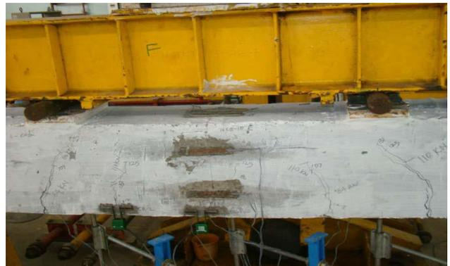
(f) final cracking at ultimate load
