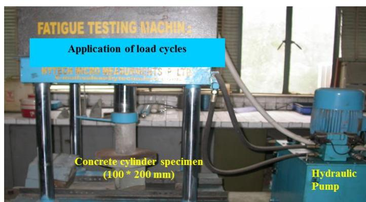
Fig. 5 – Fatigue testing arrangement
