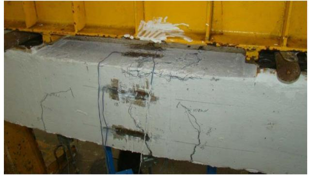
(b) final cracking at ultimate load
