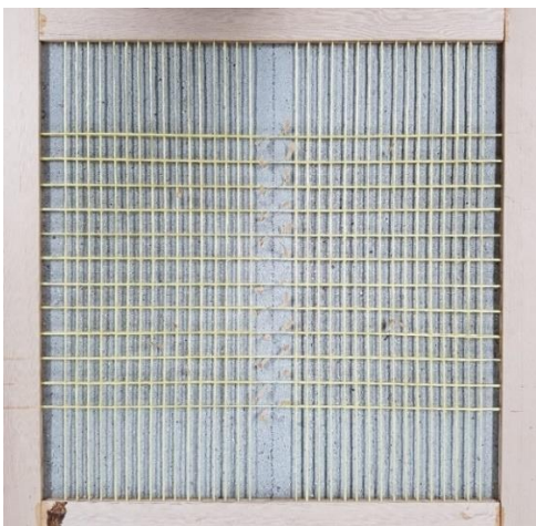
(a) AF mesh installed on top of concrete block prior to mortar casting
