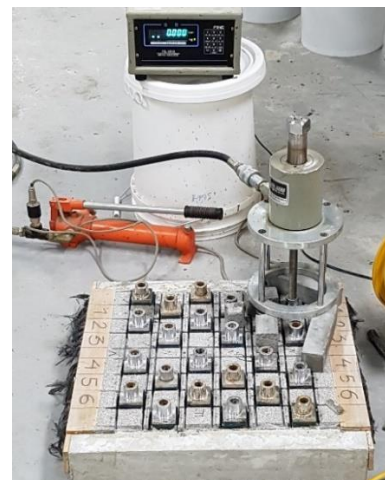
(b) Pull-off test in progress
