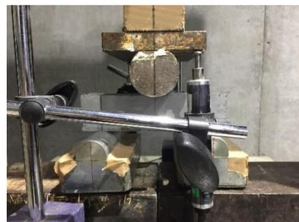
Fig. 3 – Three-point flexural test setup
