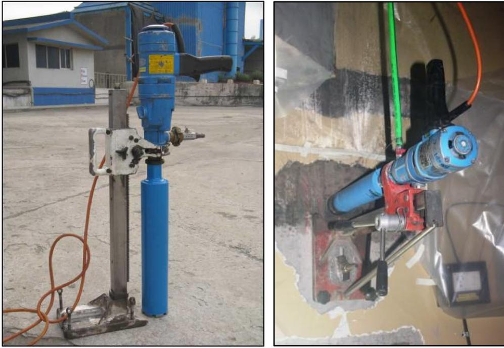
Fig. 3 – Extraction of concrete cores: (a) machine, (b) execution
