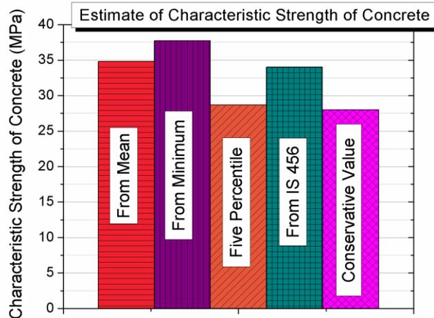
Fig. 16 – Conservative Characteristic Strength of Concrete from NDT
