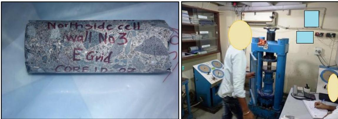
Fig. 4 – Testing of concrete cores: (a) extracted concrete core sample, (b) testing setup for compressive strength of cores
