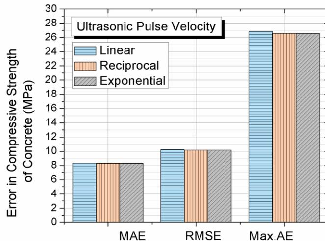
Fig. 8 – Comparison of errors in estimate of compressive strength of concrete with different equation forms for USPV-compressive strength
