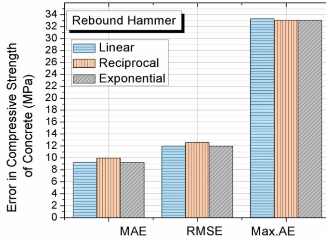
Fig. 9 – Comparison of errors in estimate of compressive strength of concrete with different equation forms for RH-compressive strength
