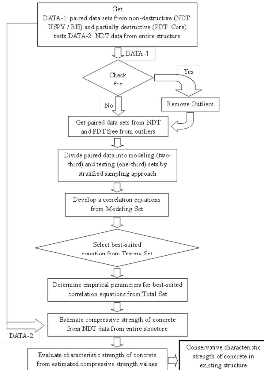
Fig. 5 – Flow-chart for the strategy for determination of conservative characteristic strength of concrete from NDT results
