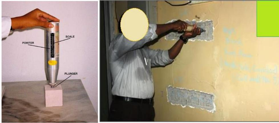
Fig. 1 – Rebound hammer: (a) machine, (b) execution
