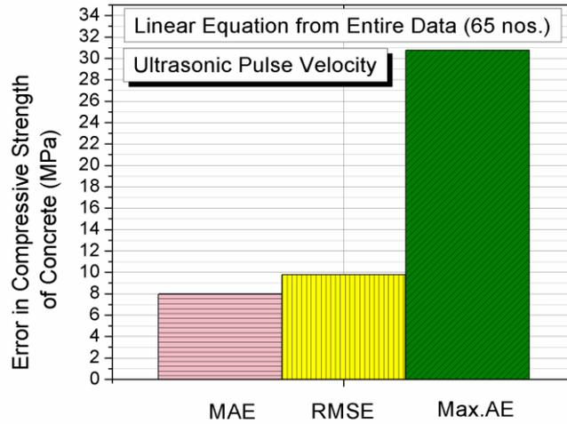
Fig. 10 – Errors in estimate of compressive strength of concrete from USPV
