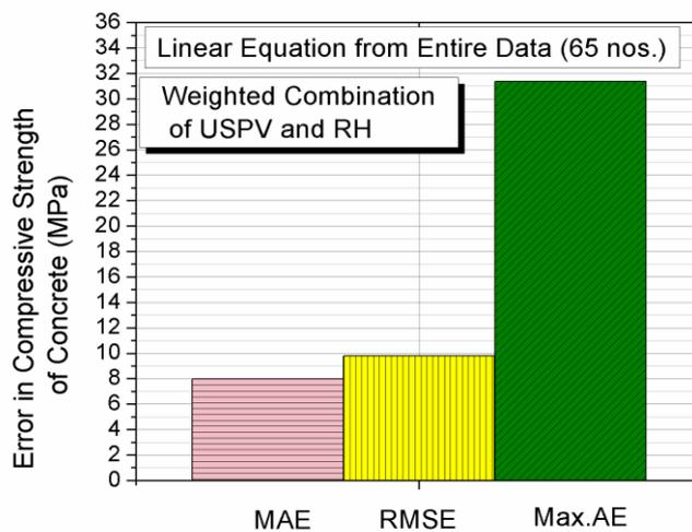
Fig. 12 – Errors in estimate of compressive strength of concrete from weighted combination of USPV and RH
