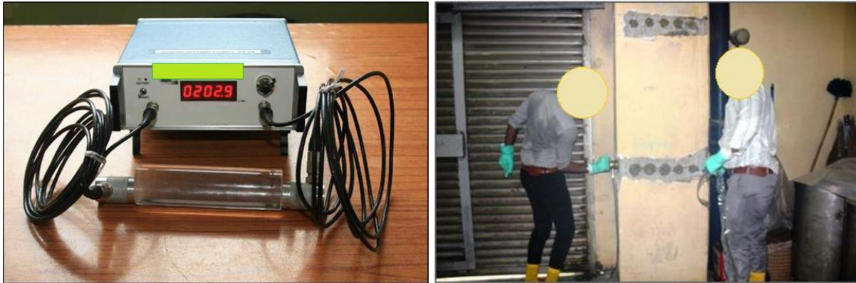
Fig. 2 – Ultrasonic pulse velocity: (a) machine, (b) execution
