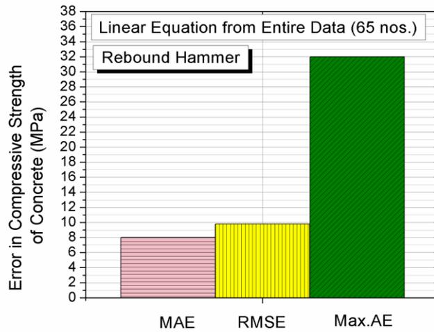
Fig. 11 – Errors in estimate of compressive strength of concrete from RH
