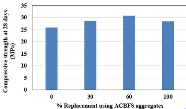
Fig. 5(a) –Compressive strength (28 days) of mixes with different replacement percentages of ACBFS aggregate
