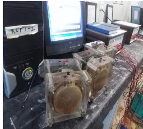
Fig. 6(a) – DC voltage system for RCPT tests
