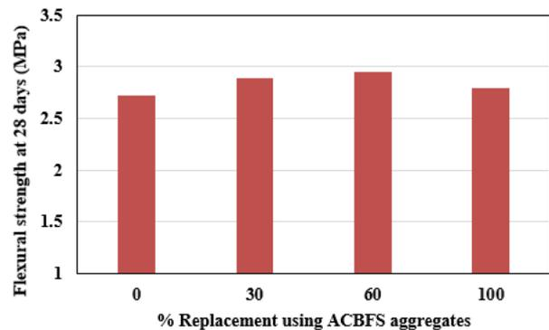
Fig. 5(b) –Flexural strength (28 days) of mixes with different Replacement Percentages of ACBFS aggregate
