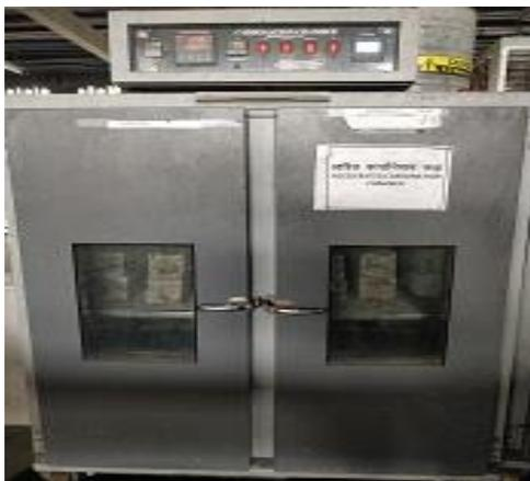
Fig. 7 – Carbonation Chamber for ACT
