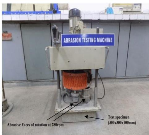
Fig. 9 – Revolving-disk abrasion test machine
