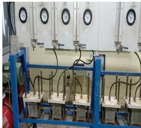
Fig. 8 – Test Setup for Water permeability test
