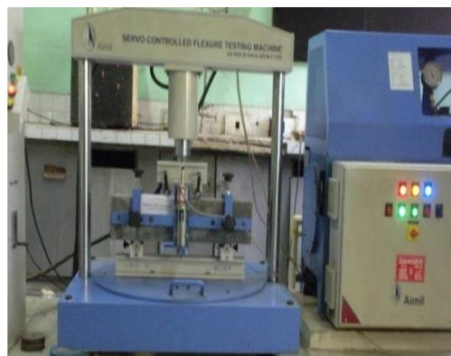
Fig. 2 – Sample undergoing Flexural Strength Test
