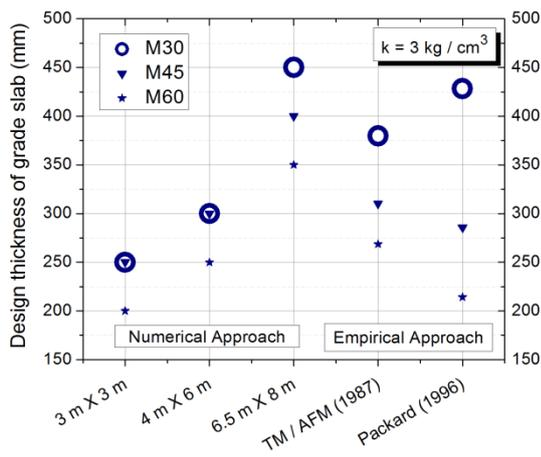
Fig. 6 – Comparison of design thickness of grade slab by empirical and numerical approaches for modulus of sub-grade reaction = 3 kg/cm<sup>3</sup>
