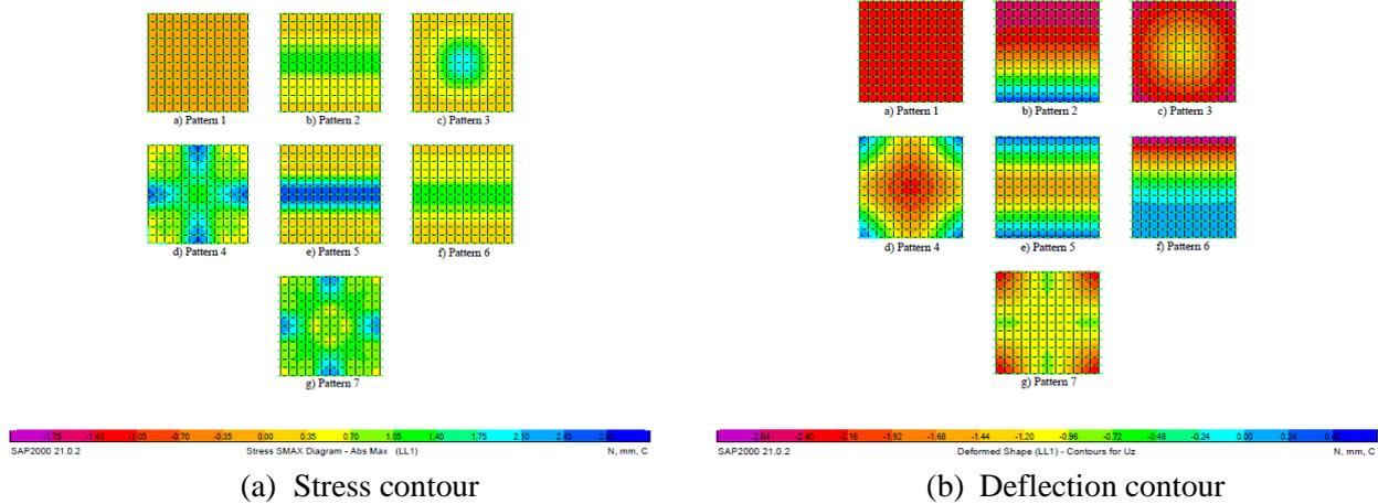
Fig. 2 – Contours for different loading patterns (modulus of sub-grade reaction of 3.00 kg/cm<sup>3</sup>)
