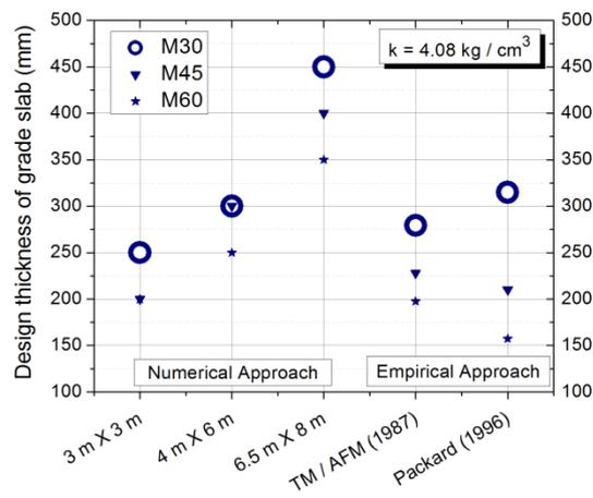
Fig. 7 – Comparison of design thickness of grade slab by empirical and numerical approaches for modulus of sub-grade reaction = 4.08 kg/cm<sup>3</sup>
