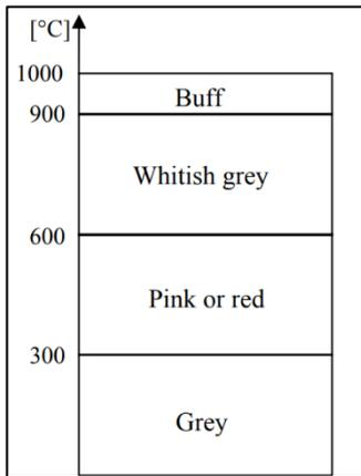
Fig.10 – Colour changes in heated concrete (fib 2008)
