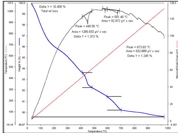
Fig.16 – DTA curve for 3rd floor corridor column (unaffected by fire) at 7-12 mm depth wherein peak due to decomposition of  $\text{Ca}(\text{OH})_2$  is present
