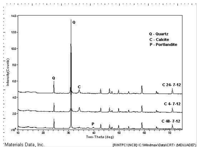
Fig.24 – XRD images of samples from C48 (3<sup>rd</sup> floor column), C24 (2<sup>nd</sup> floor column) and C4 (5<sup>th</sup> floor column) from in depth range of 7-12 mm
