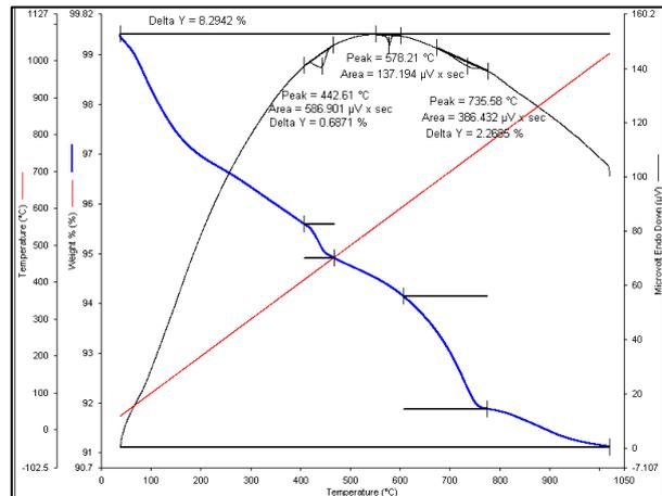
Fig.18 – DTA curve for 2nd floor column outside room where fire was first spotted at 21-26 mm depth
