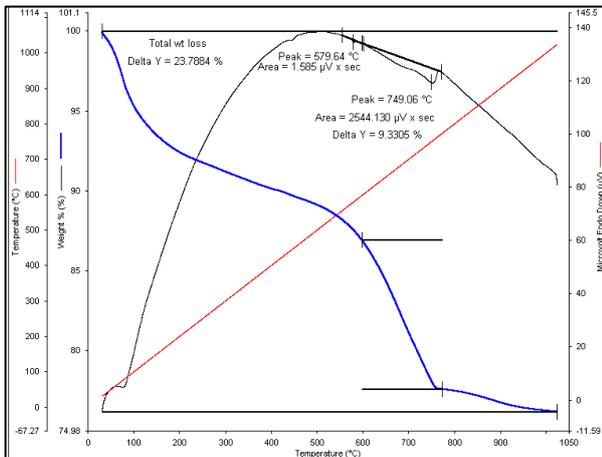
Fig.17 – DTA curve for 2nd floor column outside room where fire was first spotted at 14-19 mm depth
