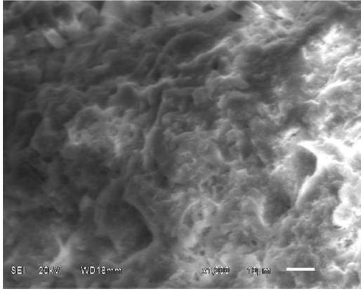
Fig.21 – SEM images of samples from 2nd floor column, from depth range of 14-19 mm depth. Presence of hexagonal morphology indicating the probable presence of portlandite
