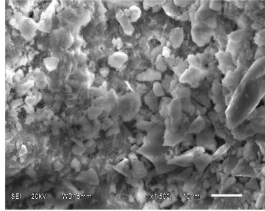
Fig.22 – SEM images of samples from 2nd floor column, from depth range of 21-26 mm depth. Hexagonal morphology is absent. Microstructure found to be less densified with presence of micro pores and micro cracks
