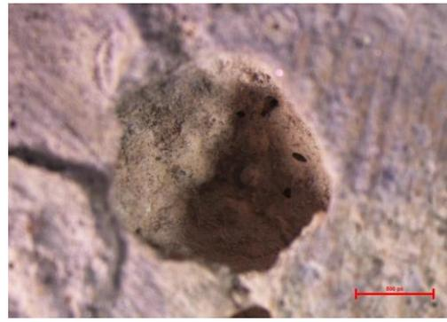
Fig. 28 – Development of micro cracks at the base of void from fire damaged concrete (15X)
