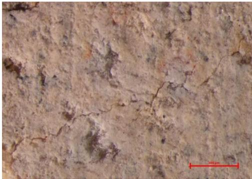
Fig. 29 – Formation of micro cracks in cement mortar and at the interface of aggregate and cement mortar (45X)
