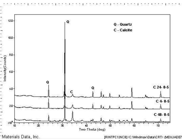
Fig. 23 – XRD images of samples from C48 (3<sup>rd</sup> floor column), C24 (2<sup>nd</sup> floor column) and C4 (5<sup>th</sup> floor column) from in depth range of 0-5 mm
