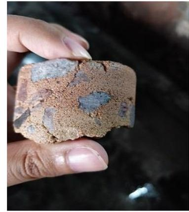
Fig.12 – Change in colour of concrete at locations close to the room where fire was first detected
