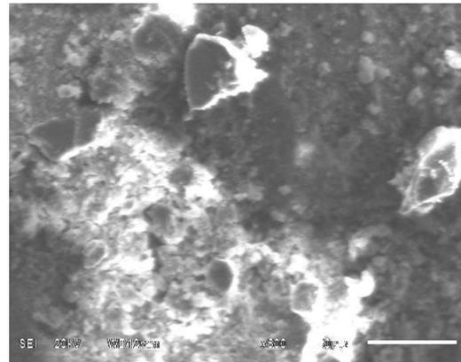
Fig.20 – SEM images of samples from 3<sup>rd</sup> floor column, from in depth range of 7-12 mm Hexagonal morphology is absent. Microstructure found to be relatively less densified and porous
