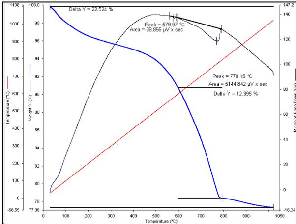
Fig. 15 – DTA curve for 3rd floor corridor column (unaffected by fire) at 0-5 mm depth wherein peak due to decomposition of  $\text{Ca}(\text{OH})_2$  is absent – due to carbonation
