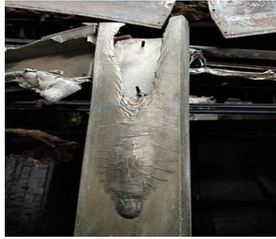
Fig. 2 – Localized softening and partial melting of Aluminum
