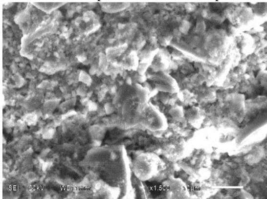
Fig.19 – SEM images of samples from 3<sup>rd</sup> floor column, from in depth range of 0-5 mm. Hexagonal morphology is absent. Microstructure found to be relatively less densified and porous
