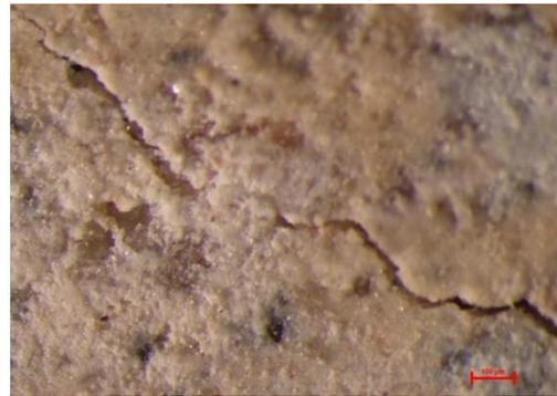
Fig. 30 – Formation of micro cracks in cement mortar and at the interface of aggregate and cement mortar (90X)
