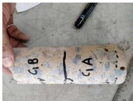
Fig.14 – Demarcation of concrete core into two parts (A & B) for separate testing of outer and inner part
