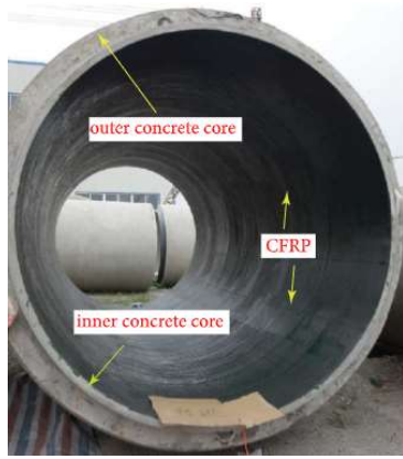
Fig. 13 – The image of CFRP-lined PCCP [85]
