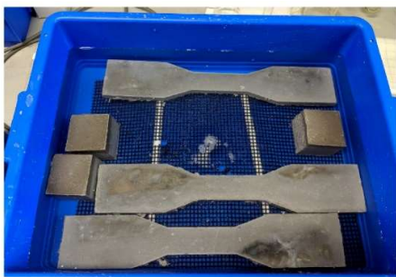
Fig. 7 – Sulfuric acid corrosion test for mortar samples (modified from [39])
