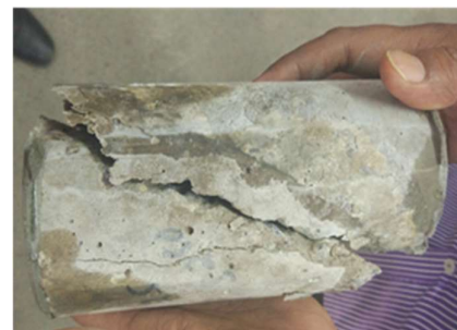
Fig. 7 – Test specimen after slant shear test
