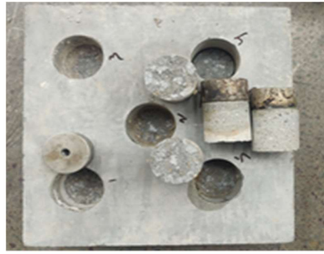
Fig. 9 –Test specimen after pull-off test
