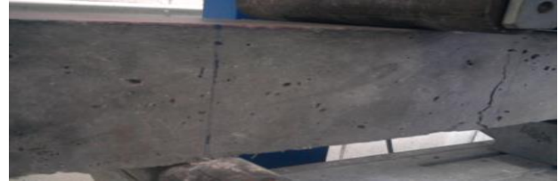
Fig. 17 – KFRC prism failure
