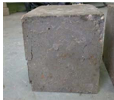
Fig. 13 – KFRC cube failure
