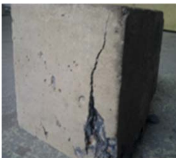
Fig. 12 – Control cube failure
