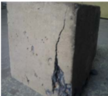
Fig. 12 – Control cube failure
