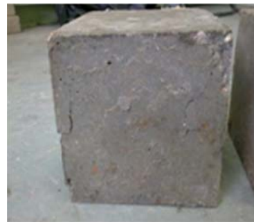
Fig. 13 – KFRC cube failure
