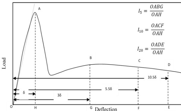
Fig. 4 – Toughness as defined by ASTM 1018
