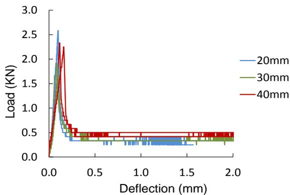
(c) Straight R-nylon fiber with 1.5% fiber fraction
