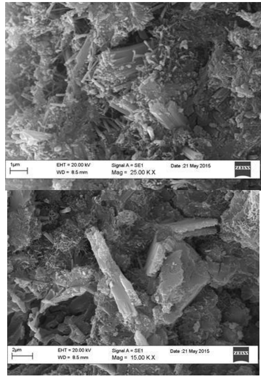
Fig. 4 – Morphology of hydration products at 3 days
