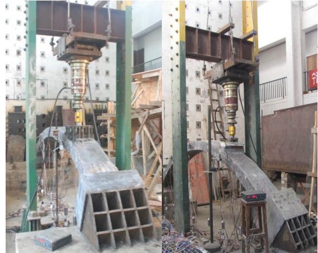
Fig. 9 – Test set-up of the UHPC arch models
