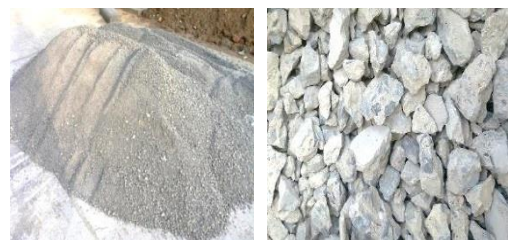
Fig. 1 – RCA particles after crushing
