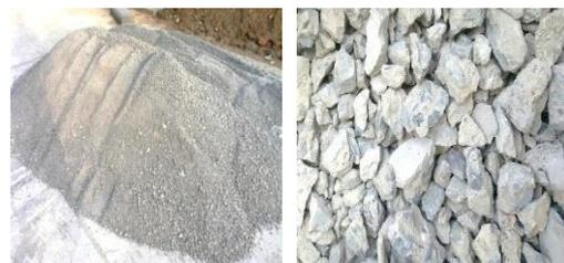
Fig. 1 – RCA particles after crushing
