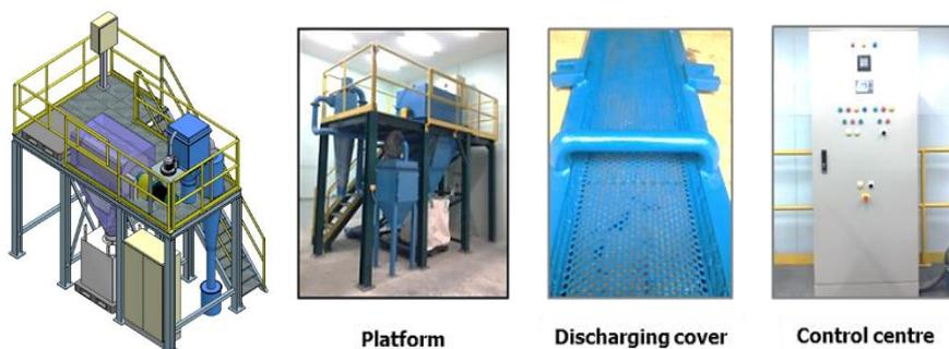
Fig. 4 – Cylindrical 500-liter rotary mill for RCA
