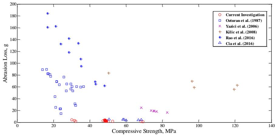
Fig. 9 – Compressive strength versus abrasion loss based on dry abrasion tests
