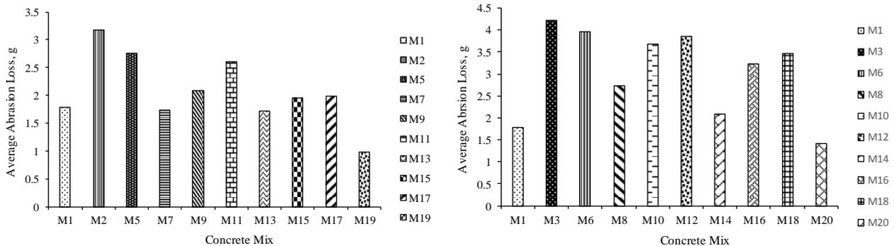
Fig. 8 – Comparison of various mixes with the bench mark mix M1
