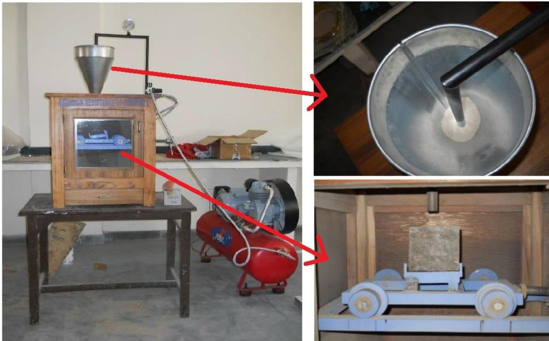
Fig. 1 – A view of sand blasting test setup
