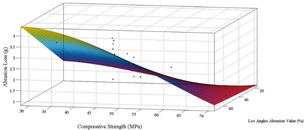
Fig. 10 – Correlations between average abrasion loss, compressive strength and L.A. value of aggregates
