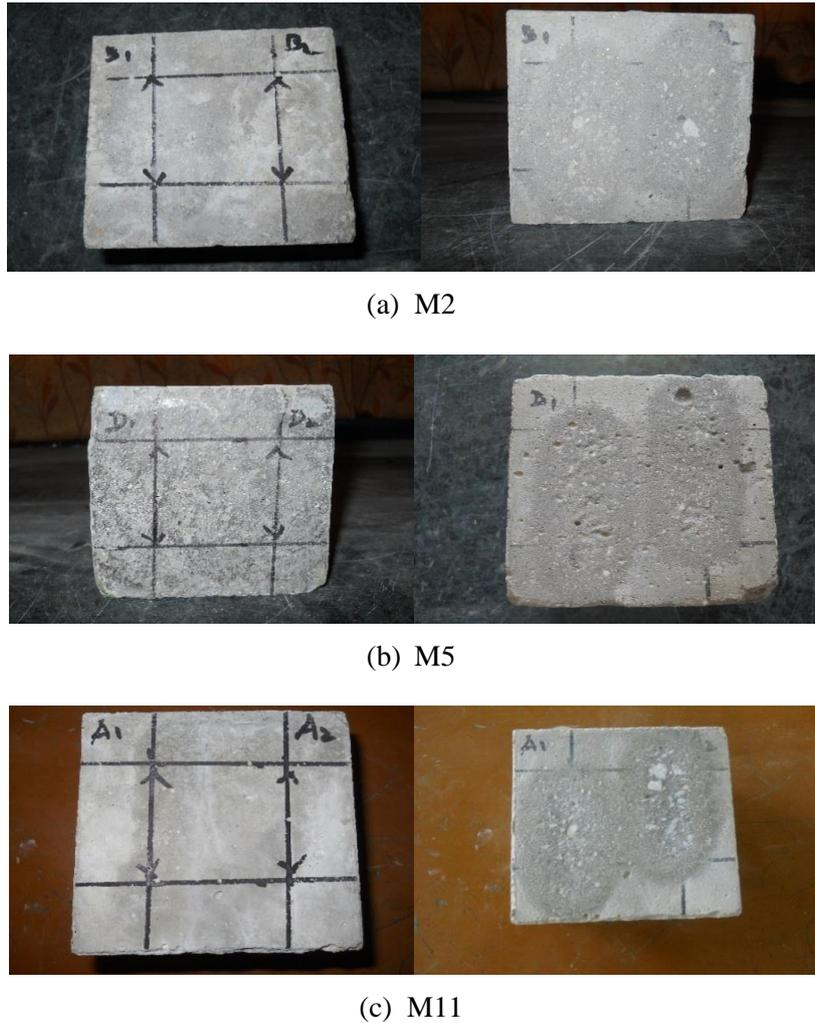
Fig. 4 – The appearance of few typical specimens before and after the abrasion resistance test by sand blasting
