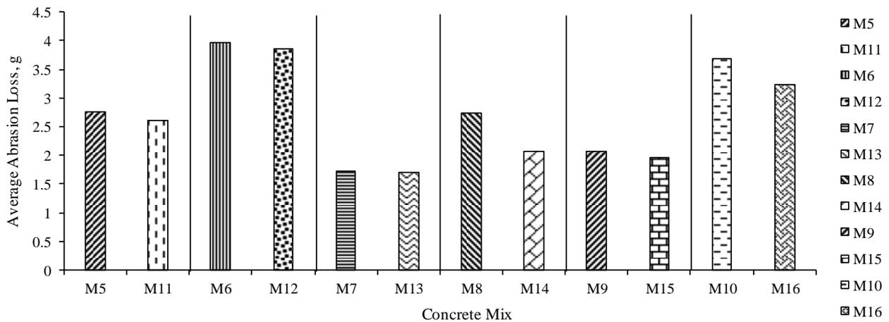
Fig. 7 – Effect of cement type on the abrasion resistance of concrete
