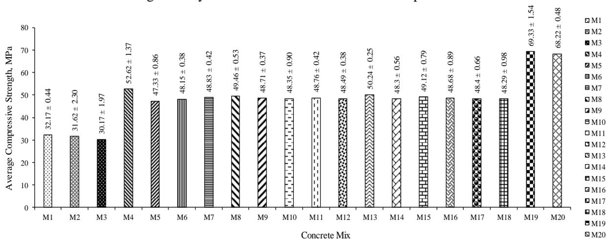
Fig. 3 – Average cube compressive strength of concrete mixes at the age of 28 days
