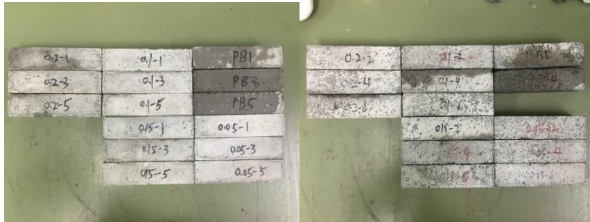
(a) Group A after 160 freeze-thaw cycles (b) Group B after 36 freeze-thaw cycles Fig. 8 – Appearance of bottom surfaces of mortar specimens
