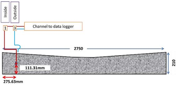
Fig. 6 – Typical arrangement of thermocouple in field measurement-1
