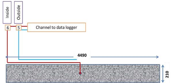
Fig. 7 – Typical arrangement of thermocouple in field measurement-2
