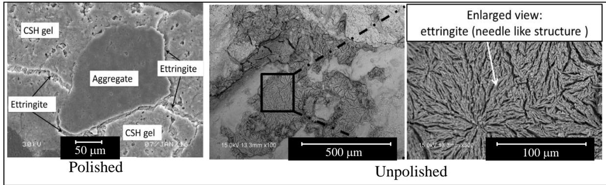
Fig. 14 – Polished and un-polished specimen: Sample D
