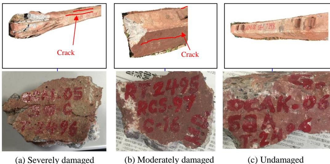
Fig. 11 – Typical concrete sample
