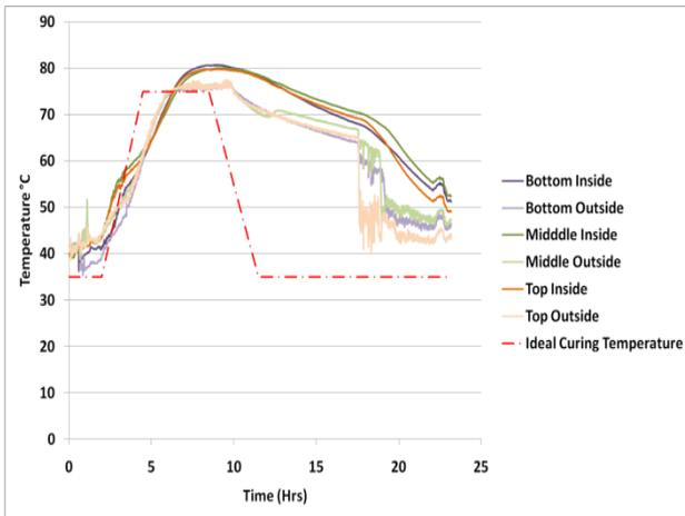
Fig. 8 – Results of temperature measurement-1 in sleeper plants in India
