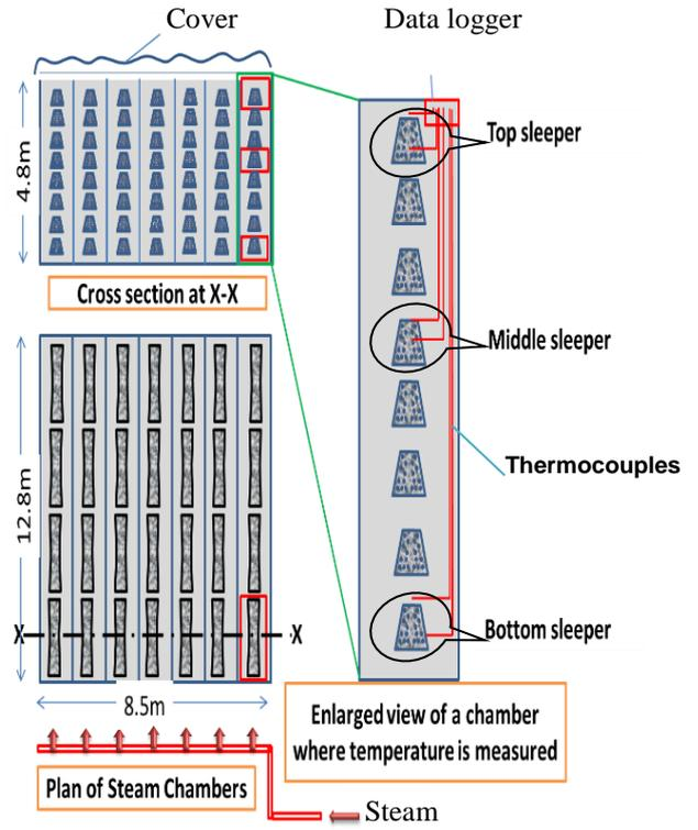
Fig. 5 – Schematic diagram of curing chambers adopted in stress bench method
