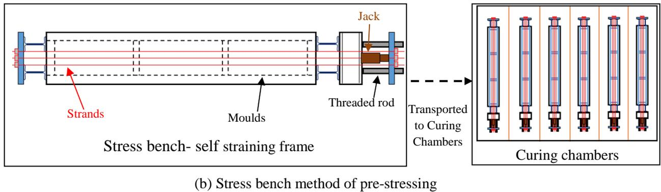
Fig. 10 – Schematic diagram showing “long line method” and “stress bench method” of pre-stressing
