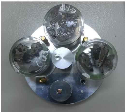
Fig. 21 – Typical specimen for EDS analysis
