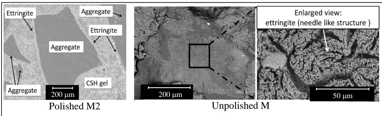
Fig. 18 – Polished and unpolished specimen: Sample M2 and M
