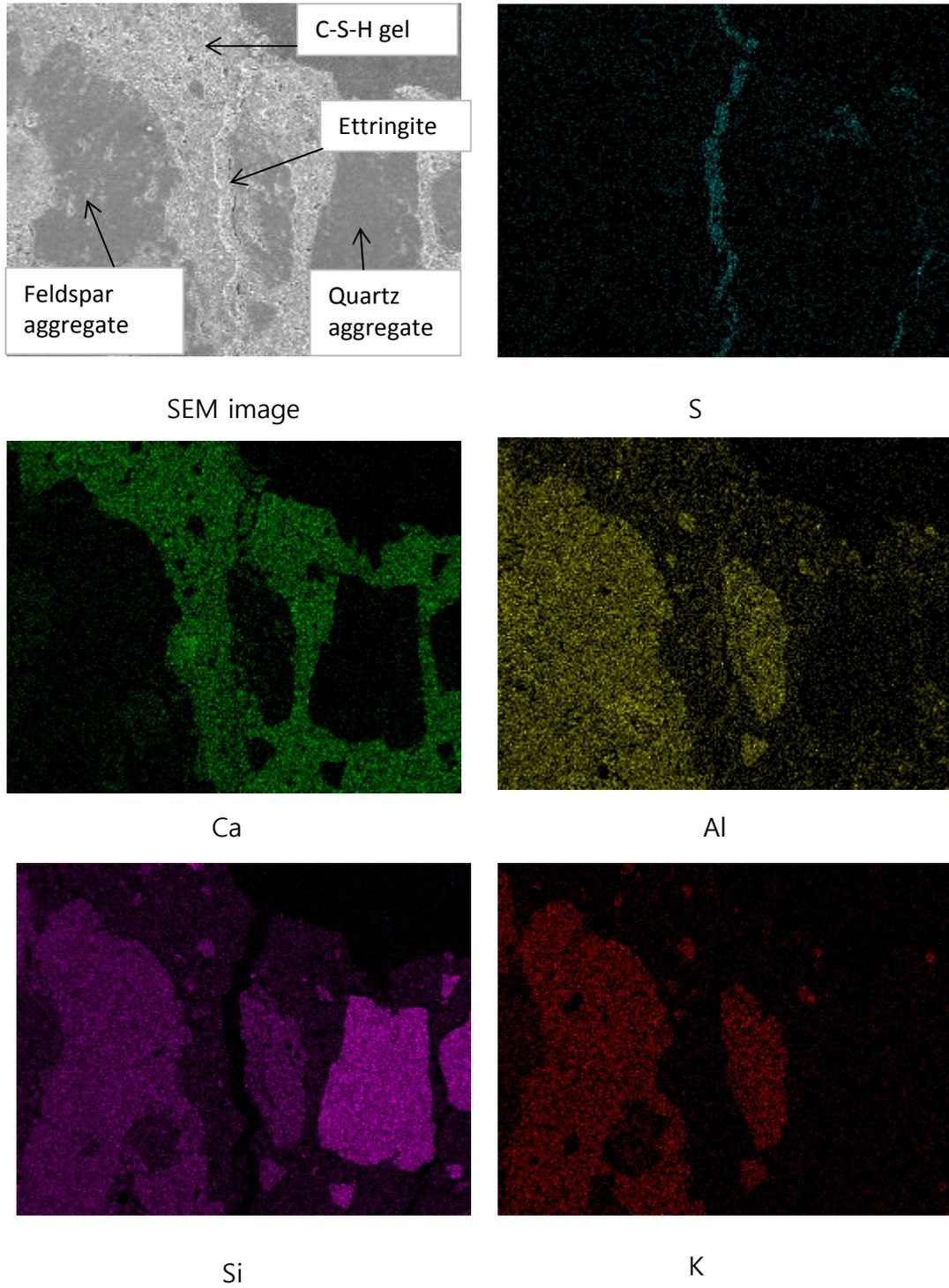
Fig. 24 – Characteristic X-ray map of sample D1
