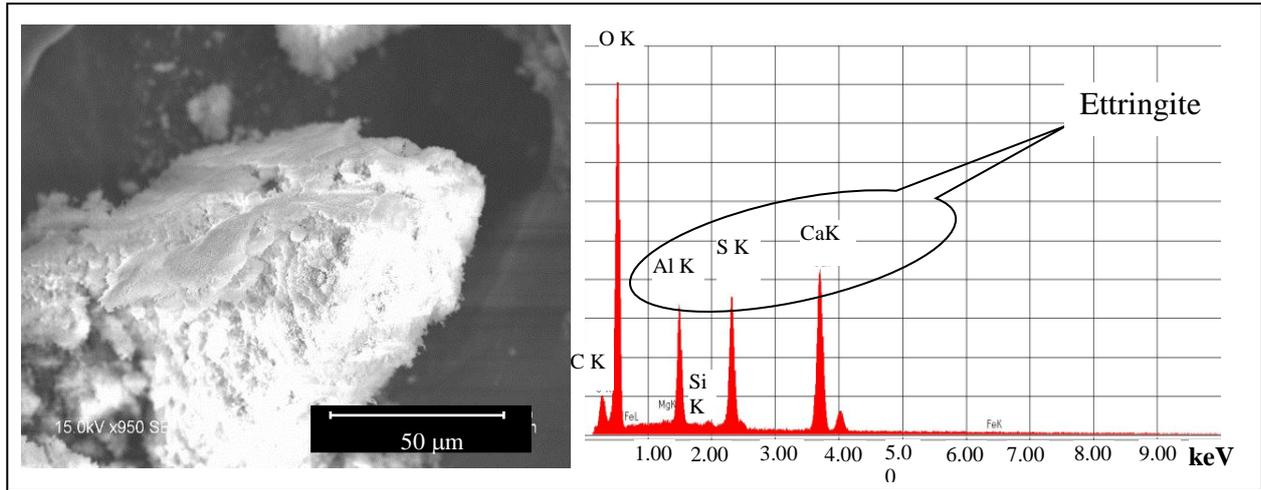
Fig. 22 – Standard synthesised specimen of ettringite
