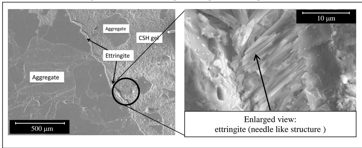
Fig. 15 – Polished specimen: Sample DU1
