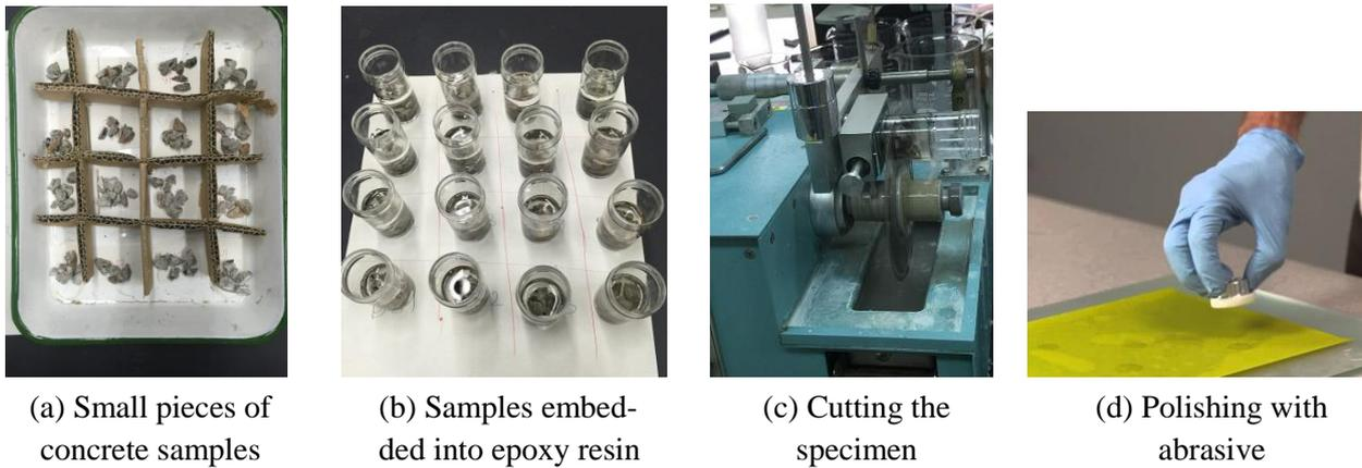
Fig. 12 – Sequence of operation for preparation of polished specimens
