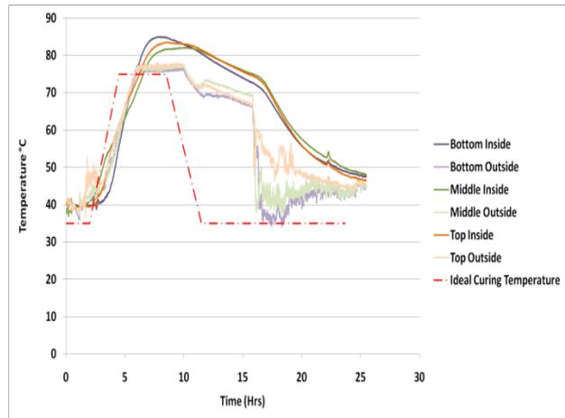
Fig. 9 – Results of temperature measurement-2 in sleeper plants in India
