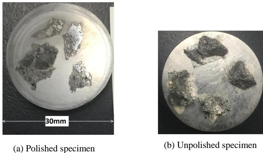
Fig. 13 – Typical Specimens used for SEM analysis
