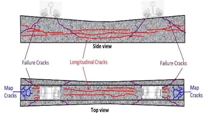
Fig. 1 – Schematic diagram of typical cracking pattern observed in concrete sleepers in Indian Railways
