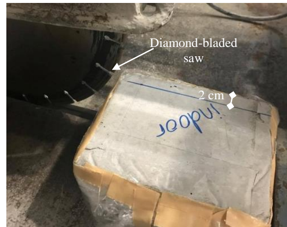
Fig. 4 – Specimen cut with a water-cooled, diamond-bladed saw
