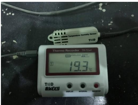
Fig. 3 – Temperature and humidity data logger
