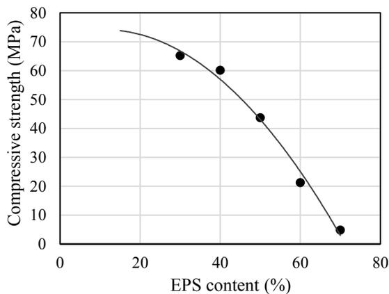
Fig. 2 – Relationship between compressive strength and EPS content by volume ratio
