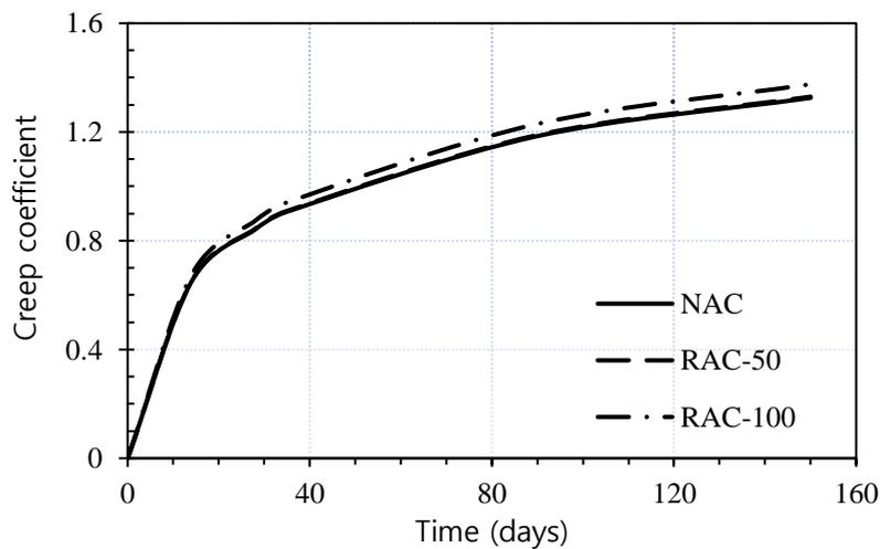
Fig. 15 – Creep coefficient prediction model by ACI 209 [29]
