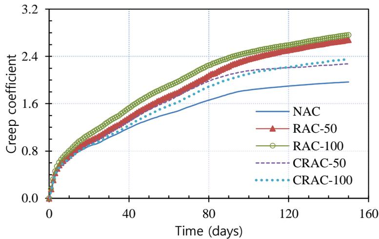
Fig. 14 – Creep coefficients vs. time after loading
