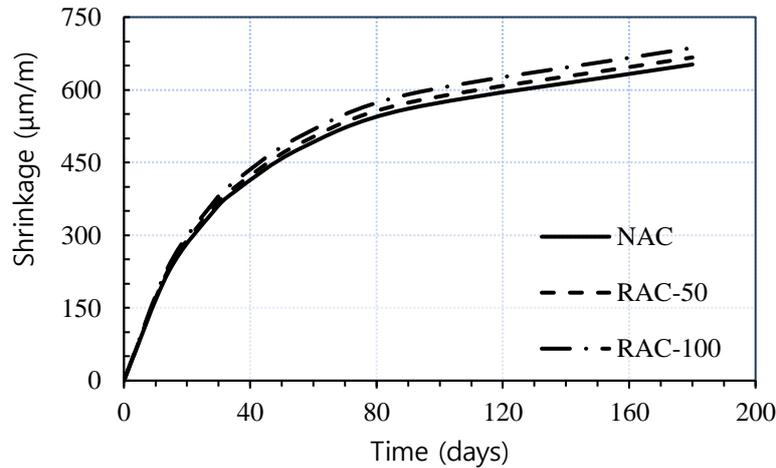
Fig. 10 – Shrinkage prediction model by ACI 209 [29]
