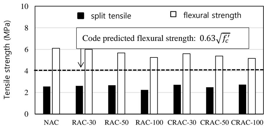
Fig. 6 – Tensile strength at 28 days
