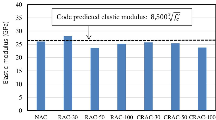
Fig. 7 – Elastic modulus at 28 days
