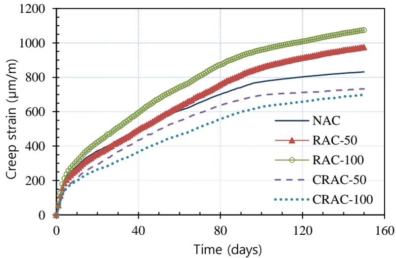
Fig. 12 – Creep vs. time after loading
