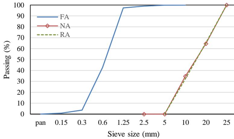
Fig. 1 – Gradation of NA, RA and FA
