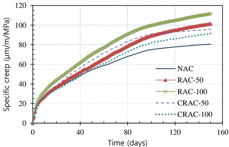
Fig. 13 – Specific creep vs. time after loading
