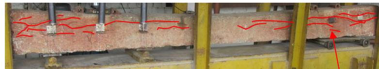
b) Severe Damaged Sleeper 3 mm cracks
