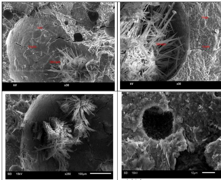
Fig. 5 – SEM images indicating ettringite in concrete samples
