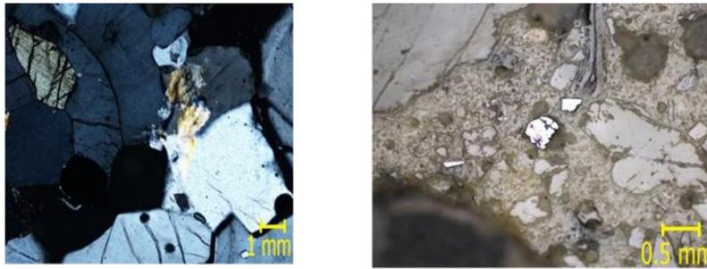
Fig. 3 – Optical microscopic images of aggregates (0.5 mm)
