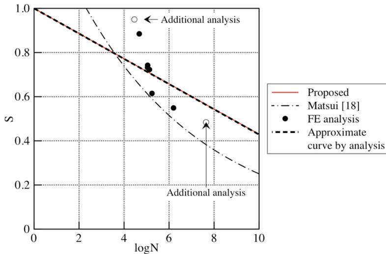
Fig. 13 – Predicted S–N curves and FE analysis results
