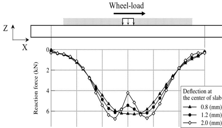
Fig. 9 – Reaction force distributions at different mid-span deflections
